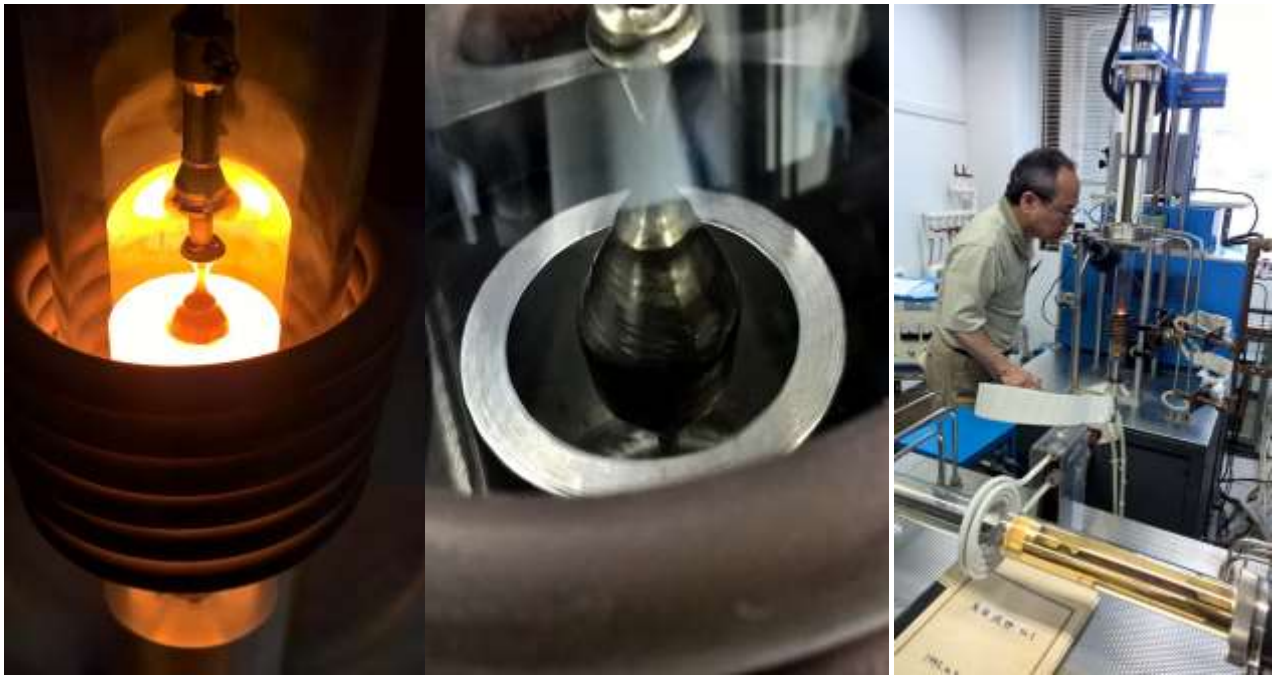
Single crystal growth of CeRh_{0.9}Pd_{0.1}Sn using the Czochralski method at Hiroshima University in Prof. Toshiro Takabatake's group. Prof. Takabatake observing the crystal growth (right)
