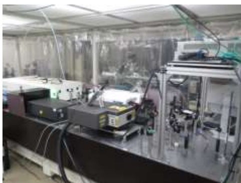
Figure 1: The femtosecond lasers used in one of the TR-PES experimental set-ups in Kyoto.
