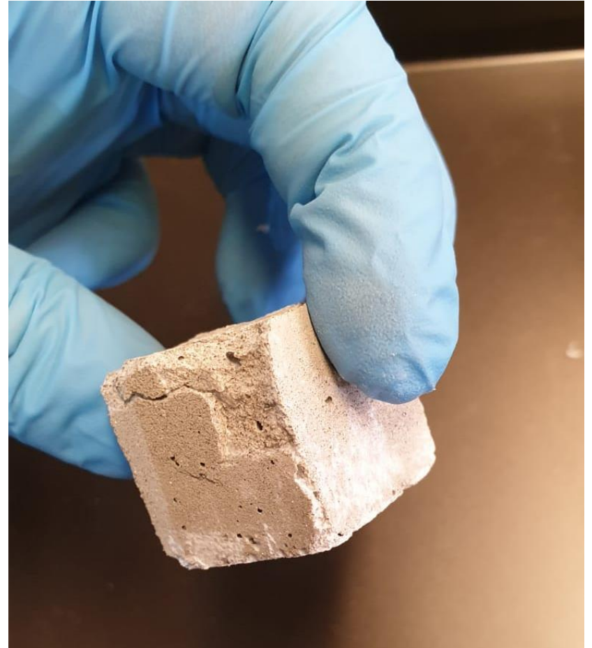
[R. Maddalena, 2019 – Cement mortar subject to freeze cycles]
