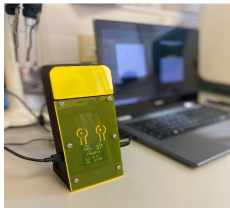
Developed portable fluorescence detector for rapid clinical diagnosis: monitoring the fluorescence signals at a constant temperature (the results will be read via a mobile App in the future)
