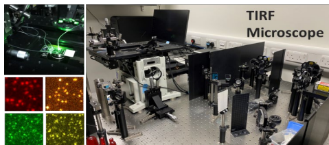
TIRF (Total Internal Reflection Fluorescence) microscope for single molecule imaging 1分子イメージング用TIRF顕微鏡
